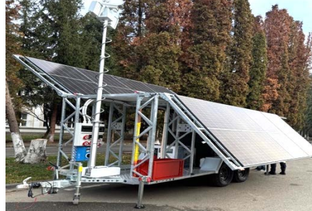
FIG. 1 MAES deployable platform with photovoltaic panels in operational position
